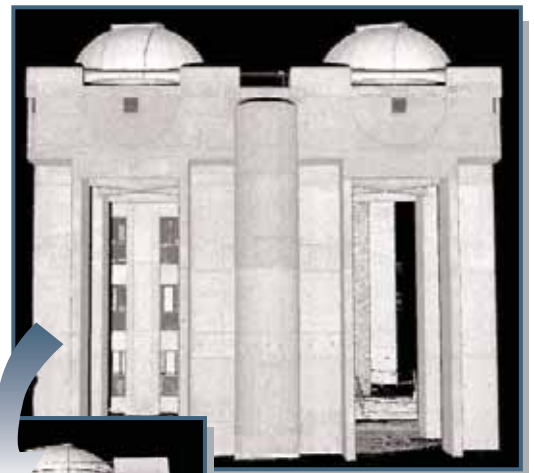
A high resolution, detailed point-cloud image was used to create a metrically accurate solid model of the building.
