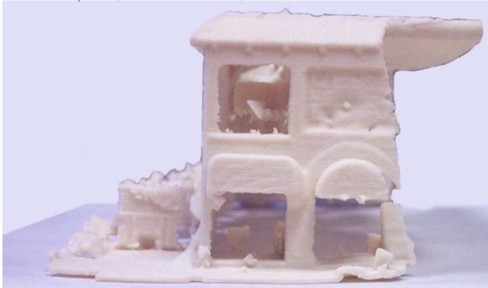
Figure 6: Rapid-prototype model of Uptown Theatre collapse (front view)
