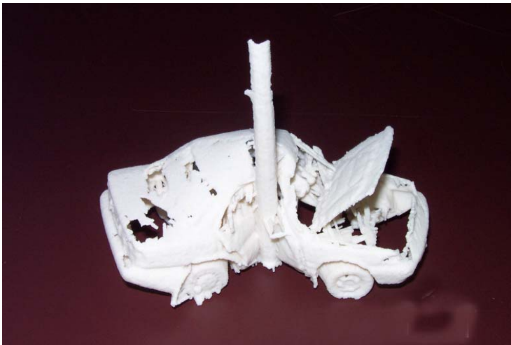
Figure 1: Rapid-prototype model of auto accident scene generated from laser scan data
